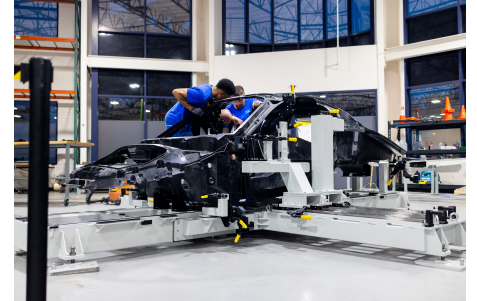
This assembly jig is used to align and bond Aptera's body structure together.
